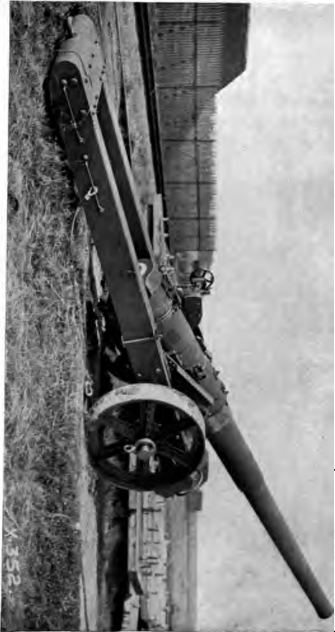
FIELD CARRIAGE FOR 6-INCH MARK VII. GUN FIRING A 20-LB. CHARGE
